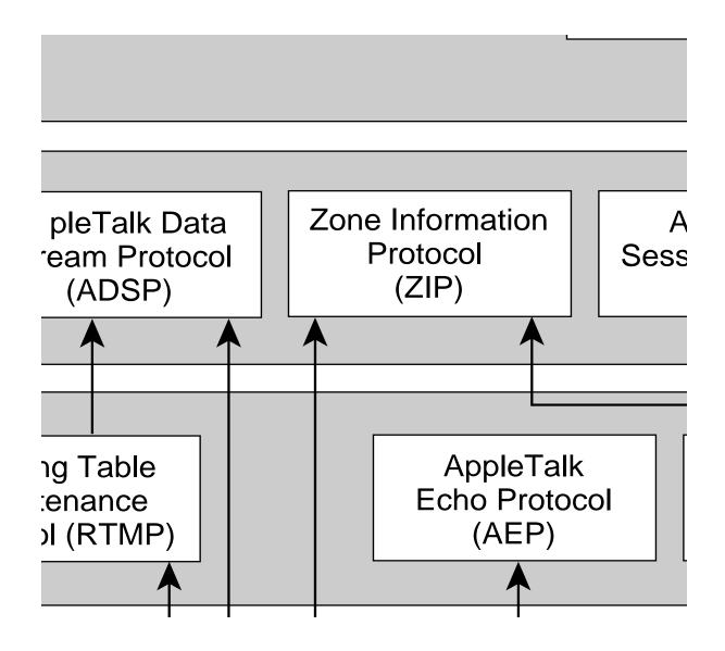
**Note:** Apple Computer uses the name "AppleTalk" to refer the Apple Networking Architecture, whereas the actual transmission media used in AppleTalk Network are referred to as LocalTalk (Apple Computer's proprietary twisted pair transmission medium for AppleTalk), TokenTalk (AppleTalk over Token Ring), EtherTalk (AppleTalk over Ethernet), and FDDITalk (AppleTalk over Fiber Distributed Data Interface).
