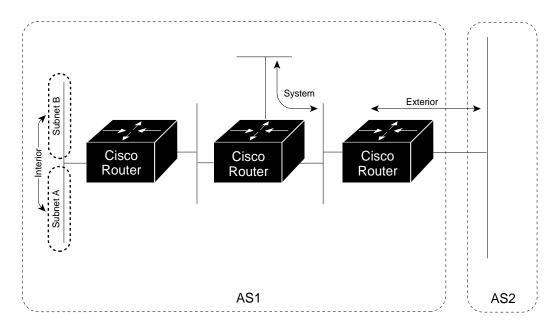
System routes are routes to networks within the autonomous system. The router derives system routes from directly connected network interfaces and system route information provided by other IGRP-speaking routers. System routes do not include subnetting information. Exterior routes are routes to networks outside the autonomous system.
