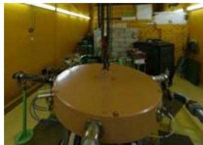
**MT-25** - Microtron electron accelerator was put into operation in 1973 (MT-17). It was totally upgraded in 1980 (MT-22) and in 1986 (MT-25). This microtron is used for study and production of ultraclean radioisotopes.
