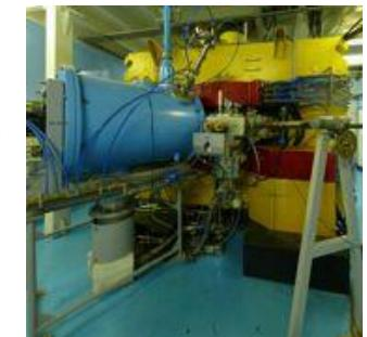
**DC-40 (IC-100)** - Cyclotron complex is the full-scale upgrade of IC-100 cycle implanter. Designed for high technology and applied research.
