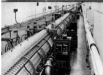
Like an entry ramp to a superhighway, this 500-foot-long linear (straight-line) accelerator at Fermilab pushes protons up to velocities needed to enter high-speed lanes in main circular accelerator. Such "preboosters" will be used in proposed 30-mile atom smasher shown above.
