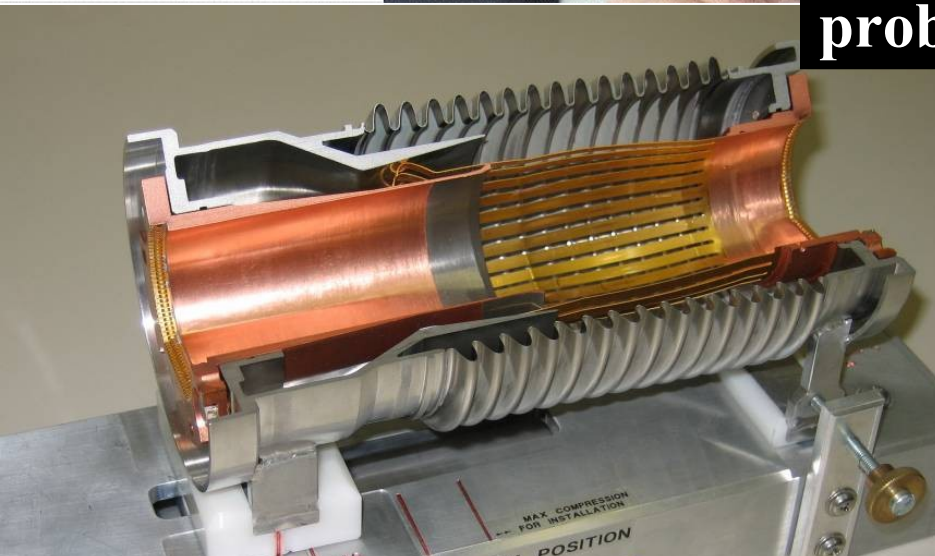
Arc plug-in module at working temperature
