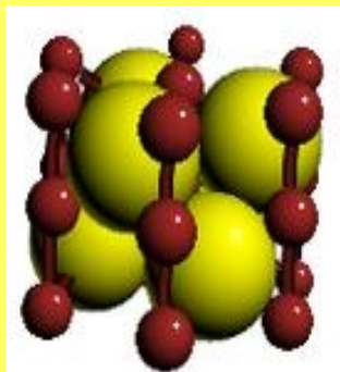
Hexagonal NiAs-type structure (P63/mmc, #194) a = 3.730 \text{ \AA} , c = 5.668 \text{ \AA} , Z=2
