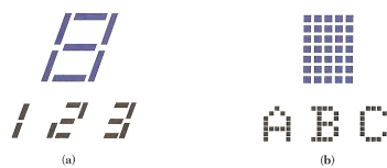
Fig. 12 LED display formats for numeric and alphanumeric: (a) 7-segment (numeric); (b) 5 × 7 array (alphanumeric). 8
