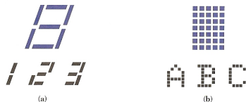
Fig. 12 LED display formats for numeric and alphanumeric: (a) 7-segment (numeric); (b) 5 \times 7 array (alphanumeric). 8
